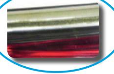
Dirt/moss can stick to the back side of the combination lamp outer edge (not inside the lamp) and can be seen through the lens, causing poor appearance.
